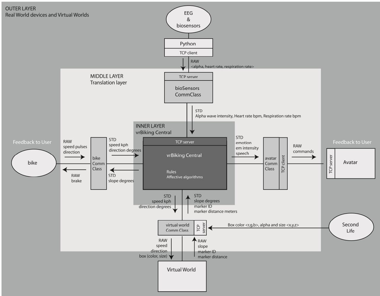
**Figure 2: Architecture of the vrBiking application.**
